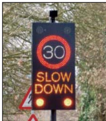
Vehicle Activated Sign which will soon be operational on School Lane
